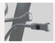
Auto-Tilt Leveling System Press the button on the hydraulic control lever to tilt the forks forward to a horizontal position. Used for easier load placement and retrieval operations.
