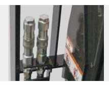
Hydraulic Quick Disconnect Simplifies change-out when multiple attachments are used to get your forklift back in operation quicker.
