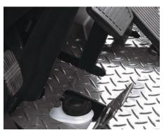
Two-piece diamond tread floorboard includes door to access brake fluid for visual level inspection and refills.
