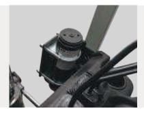
Accumulator Ideal when handling fragile loads. Feature absorbs shocks transmitted while driving over uneven or cracked floors to make load handling and travel smoother.
