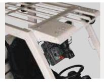
Extended Overhead Guard Extension provides protection to mounted components, including onboard computer and headlight (shown).
