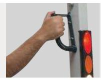
**Reverse Assist Grip with Horn** Provides operator control while driving in reverse. Keeps operator's hand securely inside the compartment during operation.
