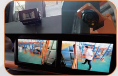
Wide field of view, all-round camera system, safer operation.
